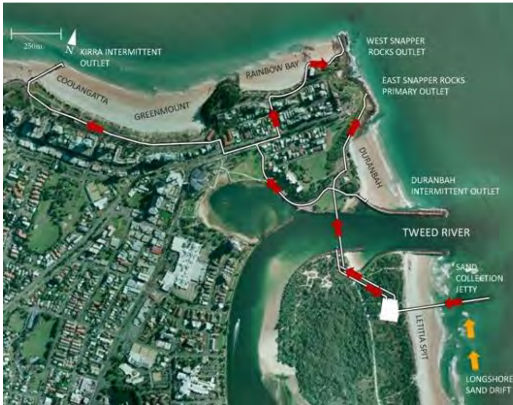
Figure 42: Schematic plan of the Tweed River Entrance Sand Bypassing Project (NSW DPI, 2016)
